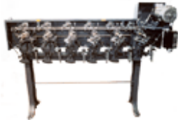
Leesona model #50 (one to twelve spindle winder) Click image for larger picture and machine description
